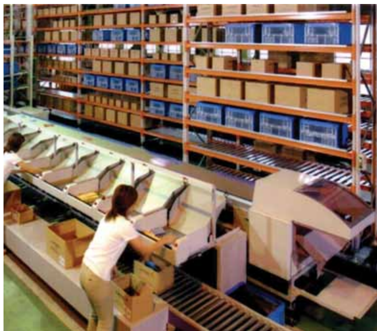
The Piece Sorter System by Daifuku can handle up to 8,000 pieces per hour
