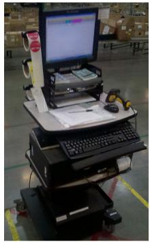
NB440 Mobile Powered Workstation with Desktop PC, LCD, Label Printer & Scanner
